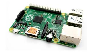
Cameras generally operate using a builtin USB cable in conjunction with a Raspberry Pi, which requires ethernet connection to the RoboRIO and power supplied from the 5V/2A terminal of the Voltage Regulator Module.
